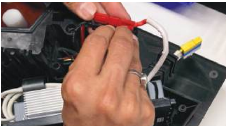
ANDERSON CONNECTOR CLIP PLACEMENT
