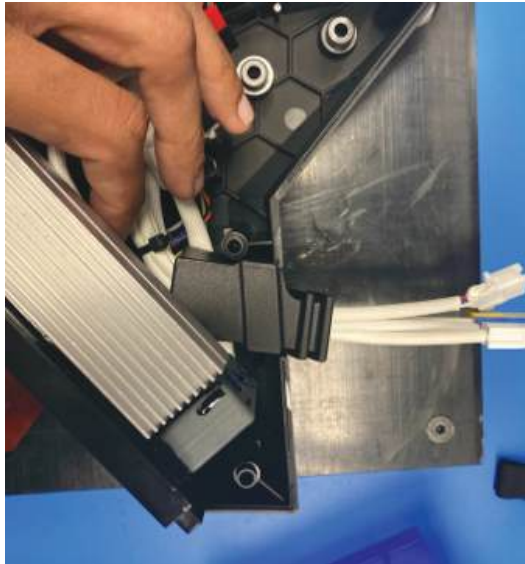
PHASE WIRES AND BATTERY PLUS/MINUS ROUTING
