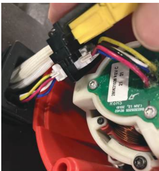
PHASE WIRES AND HALL WIRES CONNECTED
