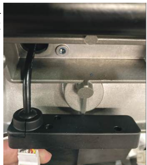
GROMMET PLACEMENT IN SUBFRAME
