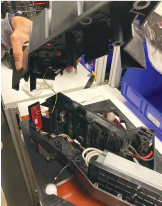
THROTTLE WIRE THROUGH SUBFRAME
