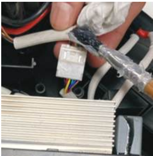
DIELECTRIC GREASE PLACEMENT
