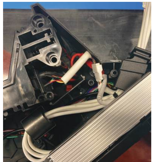
PLACEMENT OF BATTERY WIRES
