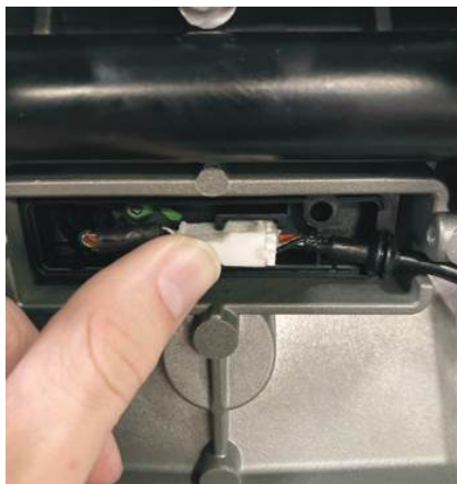
CONNECTOR HOUSING INTERNAL WIRING & PLACEMENT
