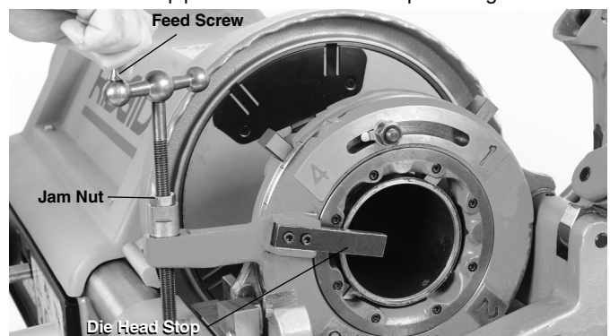
Figure 3 – Grooving the Pipe
