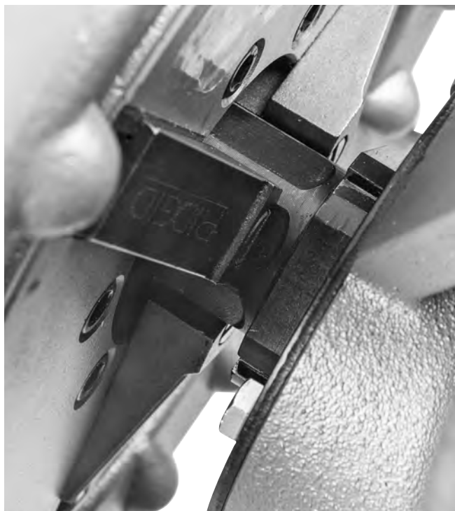
Figure 7B – Securing Drive Shaft In Chuck
