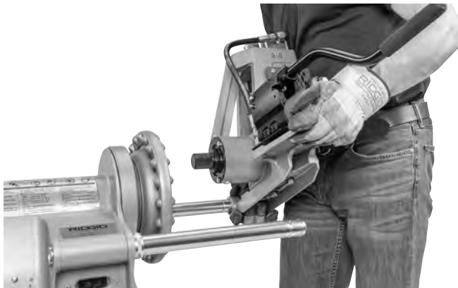
Figure 7A – Installing 918 on 300 Power Drive
