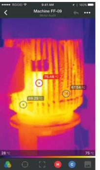
Image Detail screen allows for color palette changes, pinpoint temperature, zoom, high & low temperature and photo mode
