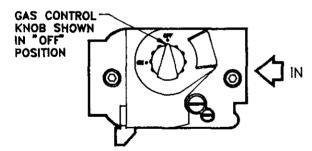
Wait five (5) minutes to clear out any gas, then smell for gas, including near the floor. If you then smell gas, stop! Follow "B" in the safety information above. If you don't smell gas, go to next step. Turn the gas control knob counterclockwise to "ON".
