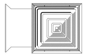
425 Series Step Down Diffuser with Slide-in Damper
