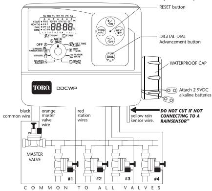
After the station wires are connected, remove the battery compartment waterproof cap and take out the two 9VDC connectors.
