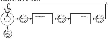
The AUTO-RUN position is used to provide information regarding the controller's operation as well as for reviewing all data stored in the irrigation programs.
